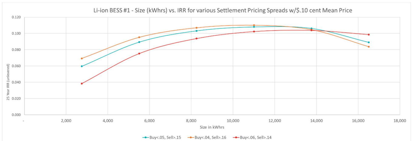
Figure 2 - The Internal Rates of Return of the Li-Ion BESS at different sizes and at 3 different pricing spreads.
